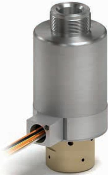
latching actuator for fire-suppression systems. The actuator accommodates operating pressures up to 300 bar, presenting the strongest actuation force for its package size. It also features fully engaged installation detection, making it compliant with NFPA 2001, Sec. 4.3.4.1 standards.
