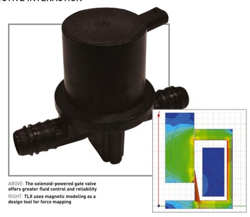
But the technology of this solenoid-powered gate valve has applications beyond SCR diesel systems. The solenoid valve can be driven by direct voltage, PWM, and peak and hold electric systems. The peak and hold signal will supply high force with smaller package sizes and lower heat generation. The smaller package size can be critical in engine applications, opening up the possibility for flow control where previous solutions would not fit.
