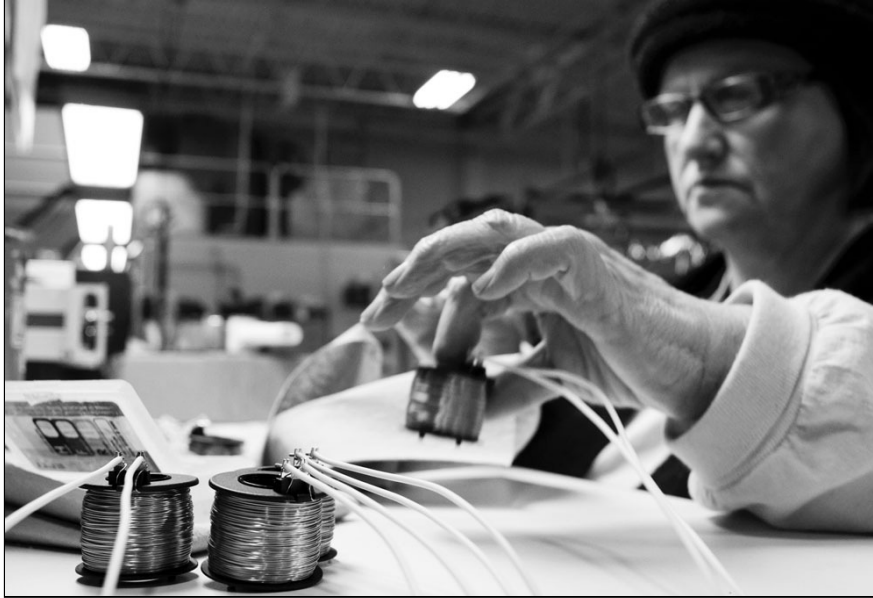
Deborah Thompson solders wires onto coils for solenoids at TLX Technologies on Wednesday.
