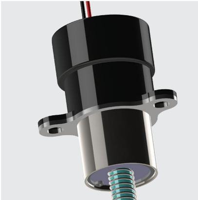
Low power draw and low heat generation have always made latching solenoids attractive, but many designers have been concerned about safety issues related to the loss of power. For example, as we just mentioned, most solenoids' armatures are held in the latched position until a reverse polarity pulse is applied. If power is unavailable, the armature can't move. The only way to prevent this is to include a failsafe system.
