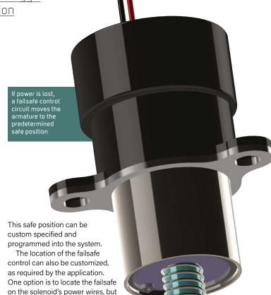
on the solenoid's power wires, but this has one significant disadvantage. If the wires are cut or damaged between the failsafe control and the solenoid, the failsafe will not function. The best and most reliable solution is to mount the failsafe directly on the solenoid. This eliminates the possibility of loss of communication between the failsafe and the solenoid should the power wires suffer damage.
