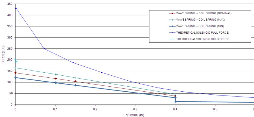
Figure 2: Typical Solenoid Force Curve
