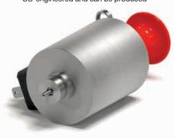
locally in the USA and China. The actuator is designed with a built-in manual override, external threads for a direct connection. and a piercing pin for a burst disk application. It also includes a safety pin to hold the piercing pin in place during pre-installation shipment. If desired, the size of the external threads and the length of the pin can be customized for your specific application. This component is durable and able to be reset for
